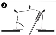
Using the handle of a hammer or screwdriver push out the speaker hood so it is fully opened and in position.
