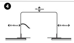
Ensure you allow a 15-20mm clearance above and a 30-40mm clearance around the fire hood.
