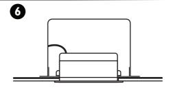
Connect the power and/or speaker cable connections prior to fixing the speaker into the ceiling.
