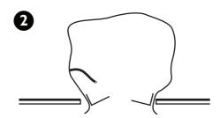
Carefully squeeze and push the speaker hood through the ceiling aperture and feed the power/speaker cable through the cable inlet.
