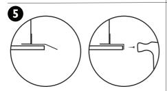
Equally space the fire hood around the aperture. Bend the 2 metal fixing strips using pliers, remove off any excess metal using cutters then screw/tack securely in position.
