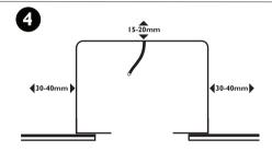
Ensure you allow a 15-20mm clearance above and a 30-40mm clearance around the fire hood.
