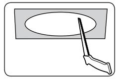
4. Insert speaker into the ceiling then using a screwdriver lock the 4 dog leg fixings to secure Attach the magnetic grille to the speaker front.
